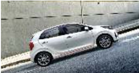
HAC (Hill-start Assist Control) At a standstill on an inline, HAC prevents you from rolling backward by gently applying the brakes, for up to two seconds, from the time you lift your foot from the brake pedal, giving you time to switch your foot smoothly to the accelerator.
