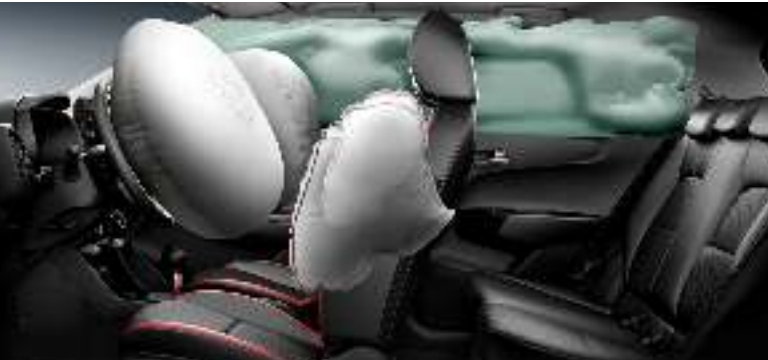
Front / side / side curtain airbags To help protect occupants and potentially reduce injuries in the event of a collision, the Picanto offers driver and front passenger airbags, two front-side airbags and two side-curtain airbags.
