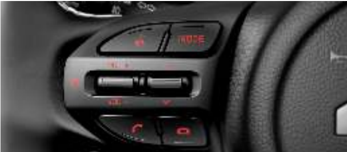
Audio remote controls Buttons mounted on the steering wheel let you adjust audio functions while your eyes stay on the road.
