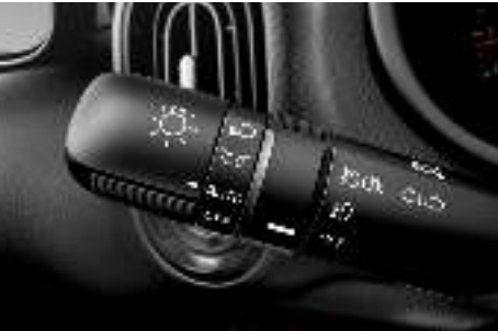
Auto light control Set the stalk ring to 'Auto' and the front and rear lights will turn on or off automatically depending on lighting conditions.
