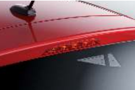
High-mounted stop lamp Located on the subtle spoiler above the rear window, the lamp safely alerts drivers behind you when you're braking.
